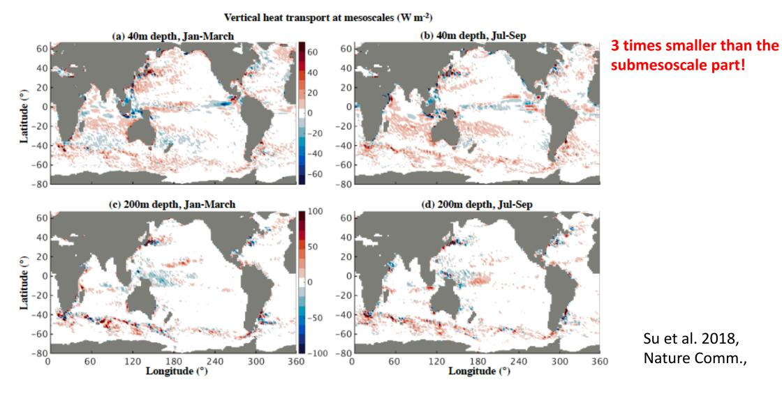
Global maps of the vertical heat fluxes in the **mesoscale band** [50 - 100 km] (W/m<sup>2</sup>).
